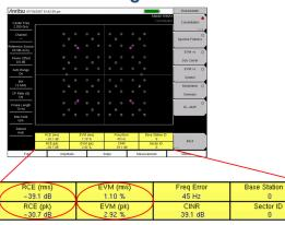
**RCE** and **EVM** measure the difference between the actual and ideal signal. RCE is measured in dB and EVM in percent.
