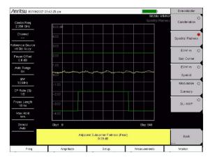
**Spectral Flatness** is a check for un-even amplitude of sub-carriers. The overall flatness measures how much BTS signal gets into of the signal is checked by the mask.
