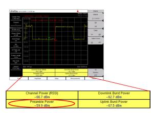
Preamble Power set cell size. A 1.5 dB change in power levels means a 15% change in coverage area. Coverage is directly affected by preamble power settings.
