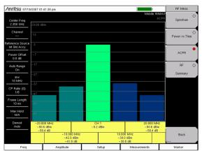
Adjacent Channel Power Ratio (ACPR) neighboring RF channels. ACPR checks the closest (adjacent) and the second closest (alternate) channels.
