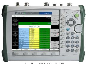
Anritsu BTS Master™ Pass/Fail screen provides status of BTS
